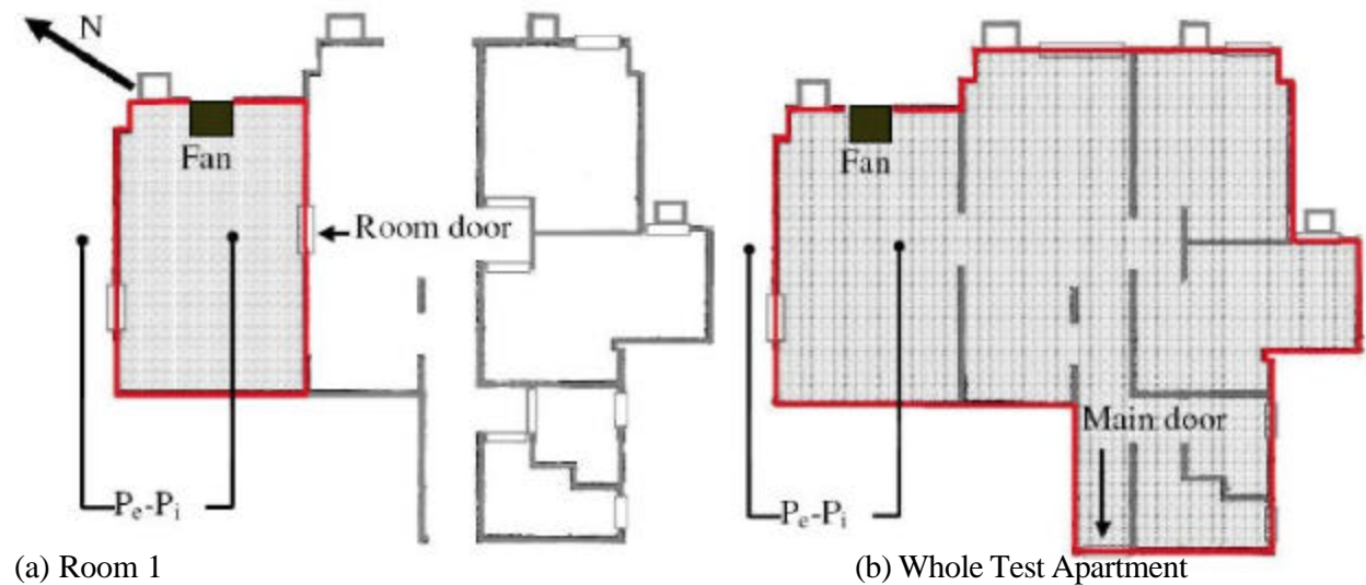
Figure 4. Configuration of permeability tests.
