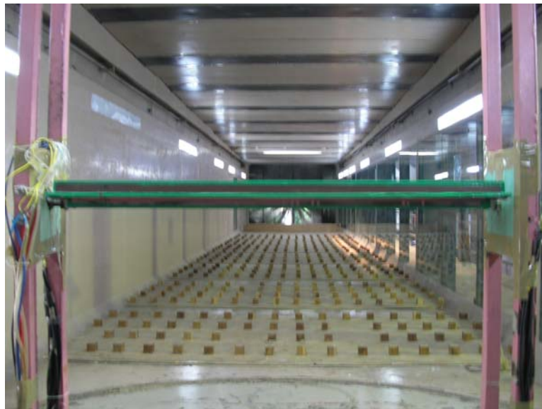
Photo 1 Test set-up inside wind tunnel for 0° wind incidence
